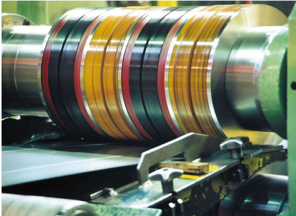
Cold rolling mill: Cold-rolled strip slitting line
