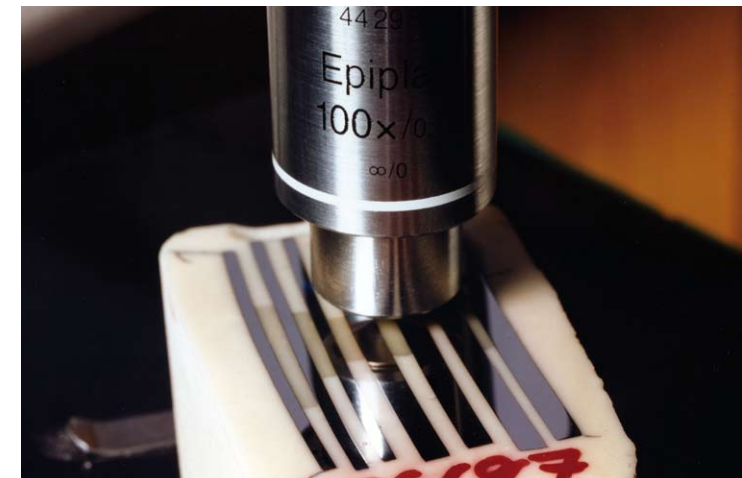
Metallographic examination of nonmetallic inclusions
