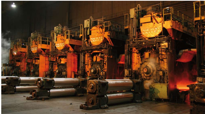
Hot rolling mill: Multiple-stand finishing group
