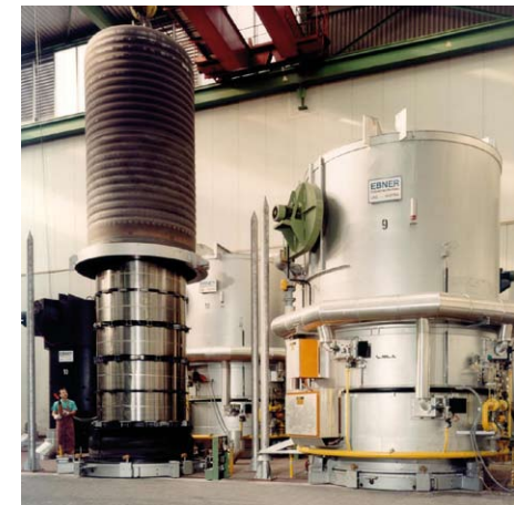
Cold rolling mill: Hydrogen high-convection batch annealing furnace
