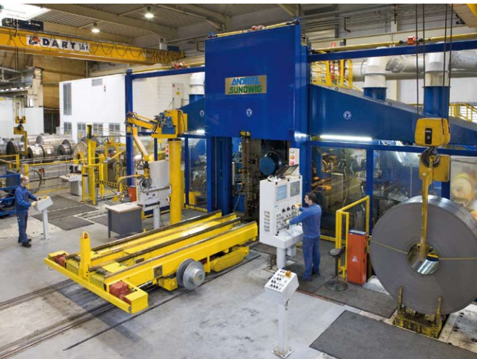
Cold rolling mill: Quarto reversing cold rolling plant
