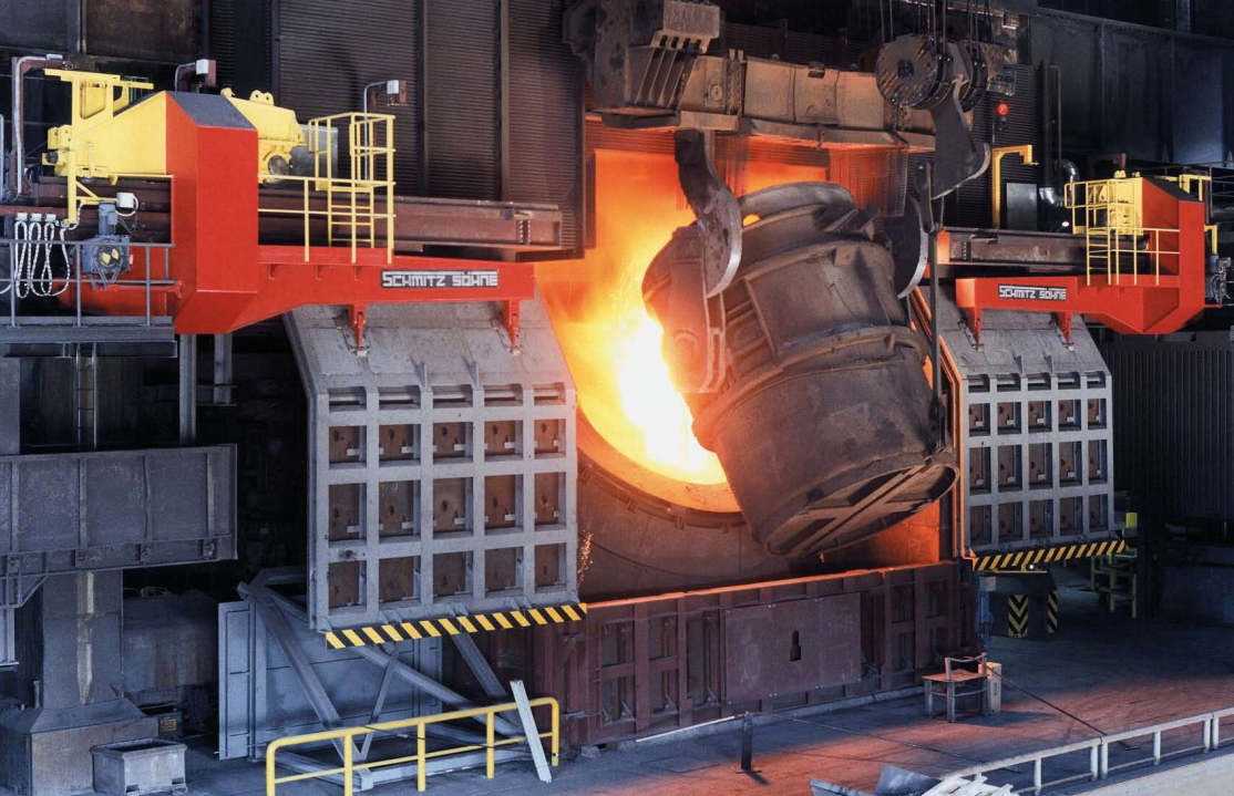
Steel plant: Oxygen converter
